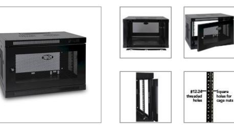
Wall-mount cabinet secures and organizes 9U of 19-inch rack equipment in network closets, classrooms and other locations with limited floor space. Houses network switches and patch panels up to 16.5 inches deep.
