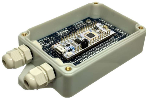
Pic. 19. IP65 Enclosure for STM DevKit
