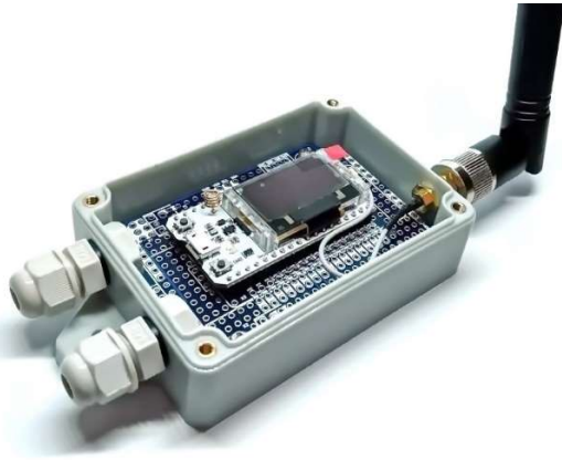
Pic. 17. WiFi LoRa controller with OLED
