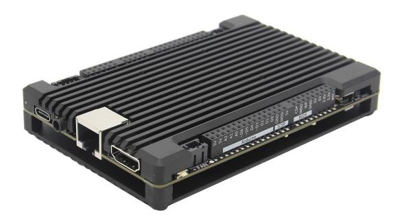
Four external fan holes are reserved on the housing, so you can conveniently add a fan on it, such as 4010, 4012 fans. (Recommended Fan Dimension:  $40 \times 40 \text{mm}$  with 32  $\pm 0.3 \text{mm}$  hole, M3 screws)
